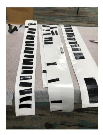
Quality check before apply Gorilla tape to ensure the staples are correct (not too many staples, 3 on each side)
